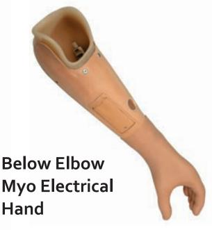
Myo Electrical arm suitable long stump user. The fingers are controlled myoelectrically, the wrists are controlled passively through mechanical rotation switch and the elbows are controlled mechanically for flexion and extension, in order to assist our user for high demanding movement such as grasping items while pronation or supination.
